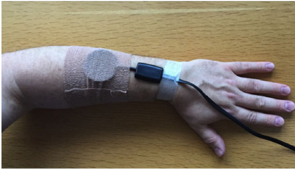
Figure 3 Typical acoustic myography recording set-up. This system only requires one sensor, unlike the three electrodes needed for surface electromyography. The sensor, which is flat, is covered on the skin side with an acoustic gel to reduce the impedance at the skin/sensor interface and then lightly held in place above the muscle of interest using a self-adhesive elastic bandage. An additional piece of tape can be used to secure the cable.
